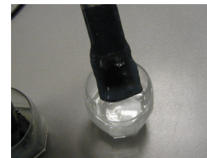
After 24 hours, the swelling of WAM 101 HD (opaque) is increased enormously, while WAM 101 WATER RESISTANT (glossy) hardly has changed the shape of the profile
