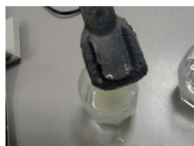
After 2 hours of immersion, WAM 101 HD (opaque) swell considerable, and WAM 101 WATER RESISTANT (glossy) does not show any change in volume
