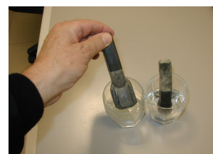
After 24 hours, the swelling of WAM 101 HD (opaque) is increased enormously, while WAM 101 WATER RESISTANT (glossy) hardly has changed the shape of the profile
